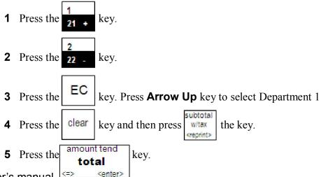
You can also use the **Arrow Up** key to scroll the clerk display, select the entry you want to void and then press the **clear** key. Press the **subtotal** key and then continue with the transaction.
