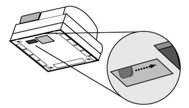
**2** Push the lever in the only direction it will move. The cash drawer opens. If the cash drawer will not open, make sure it is not locked with the 777 Drawer key.
